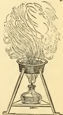
FIG. 30.—Arrangement for disengaging Sulphurous Acid Gas.
